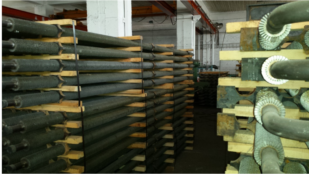
Figure 9: Finned tubes, photo from MBR Workshop at Greece
