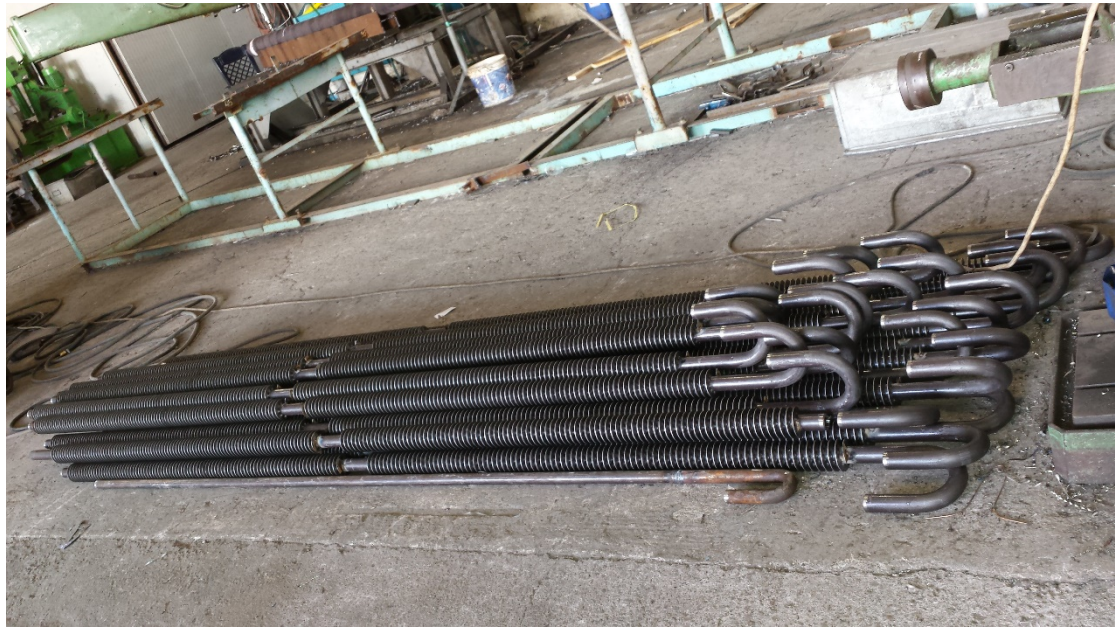
Figure 7: Spiral finned tubes, photo from MBR Workshop at Greece
